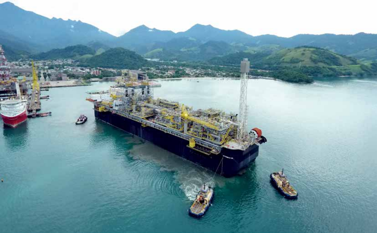
The P-66 has a production capacity of 150,000 barrels of oil/day and 6 million m 3 of gas/day
